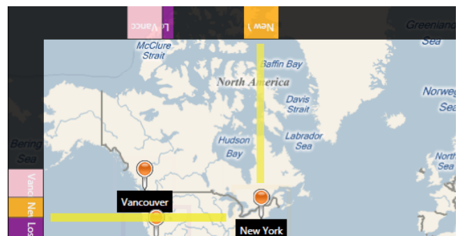
Figure 2. Edge projection. Targets are projected to the edge of the screen. Lines illustrate the correspondence between an edge proxy and its associated target.
