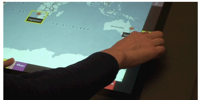
Figure 1. Access overlays allow a blind user to accurately locate items on a 2-D touch screen map.
