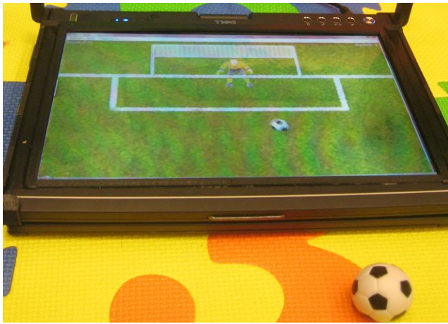
Figure 7. Penalty Shootout. The player rolls the soccer ball on the table or floor towards the screen. After the toy ball hits the tablet chassis, a virtual ball continues the physical ball's trajectory and speed towards the goal.
