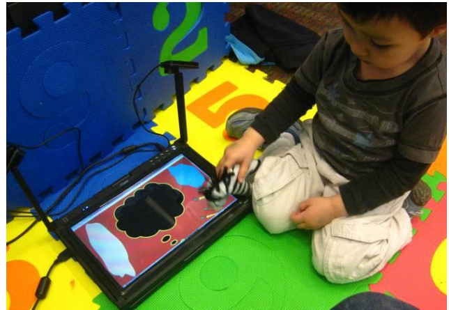
Figure 1. The Portico system in use. Two cameras track objects on the screen and surrounding surface. In this application, a toy zebra is tracked.
