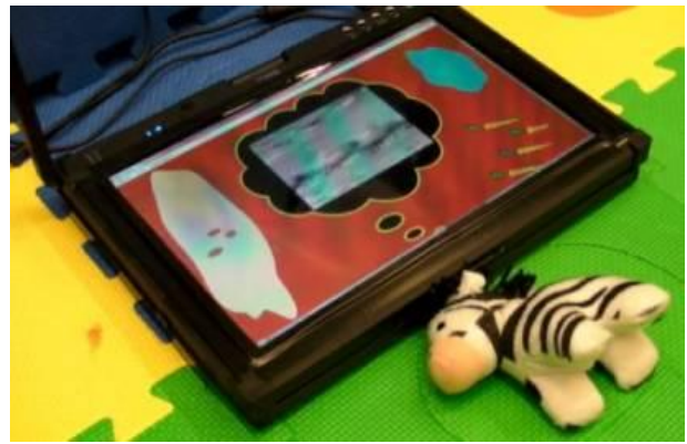
Figure 9. Tabletgotchi uses an uninstrumented zebra that “eats” carrots, “drinks” water (right side), uses the sand area (left side), or lays below the tablet and dreams (above). If the zebra stands up, the dream video stops, responding to the change in the zebra's physical state.
