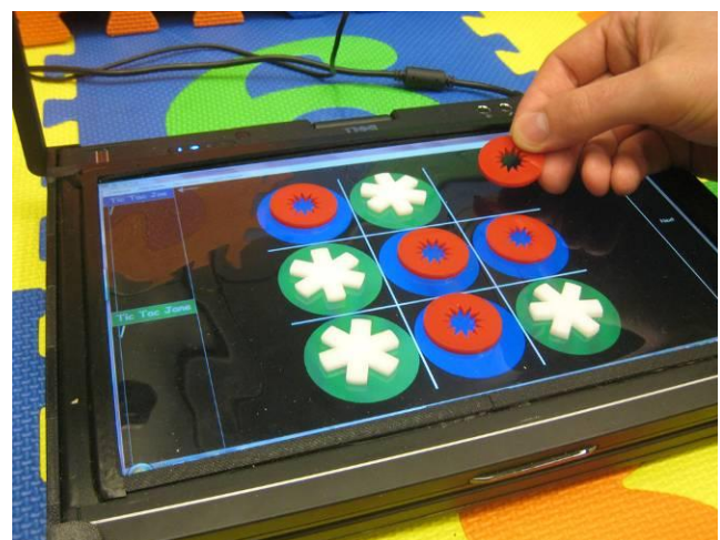
Figure 6. Using physical tokens to play Tic Tac Toe on the tablet. The game is supervised by Portico and any illegal moves are flagged (and audibly “buzzed”).
