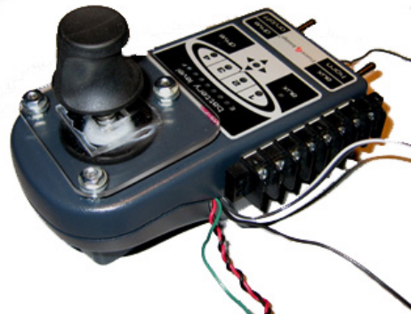
Figure 5. EdgeWrite for power wheelchair joysticks allows a power wheelchair user to enter text on their desktop computer. Note the plastic template applied to the Everest & Jennings joystick provides a square input area in which EdgeWrite letters can be made.
