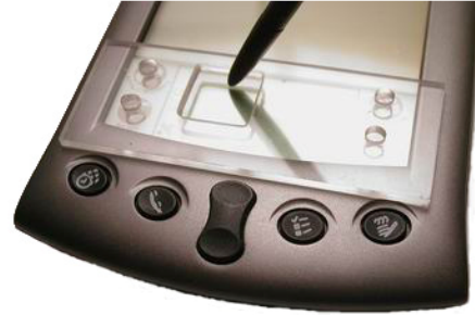
Figure 3. Our EdgeWrite template across the customary text input area on a Palm PDA. The stylus makes EdgeWrite letters by moving along the edges and into the corners of the square hole.
