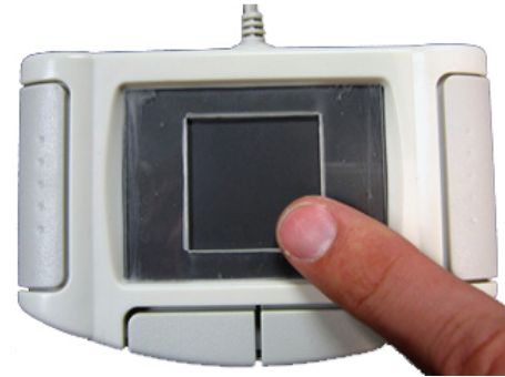
Figure 6. EdgeWrite on a stand-alone Synaptics touchpad. The finger moves along edges and into corners of the square hole in the plastic template.
