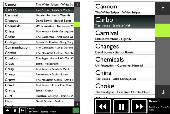
Figure 2. Our music player user interface in two sizes. (left) The player while standing; (right) the player while walking.
