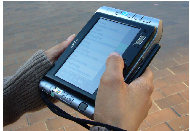
Figure 1. A participant interacting with our adaptive walking user interface (WUI) on an ultra-mobile PC.
