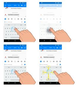
**Figure 1:** The upper figures show how rainwater interferes with sensing finger location. The water (top-left) shifts the sensed finger location to the left and down (top-right). RainCheck detects unusual capacitive signatures (bottom-left) and, among other features, offers a target selection technique to resolve ambiguity (bottom-right). In this case, RainCheck suggests a gesture (swipe) to select UI elements that were affected by the water-covered area.
