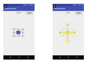
**Figure 9:** At left is the screenshot of the initial state of the task. At right is when RainCheck detected an unusual touch area and offered four potential selectable UI targets that were covered by the touch.
