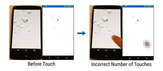
**Figure 3:** The user touches the screen with a single finger, but the touchscreen is confused due to the presence of water and detects two touch points (two red dots). However, the shape and distribution of sensor values in the finger-touch area were very different than those of water drops, giving us an opportunity for improvement.
