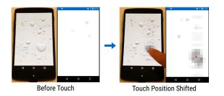
**Figure 4:** Apart from being detected as touch points, water drops also affect the center of the touch area. When the user touches a water drop and the touchscreen simultaneously (right), the touch-position extracted from the blob's center shifts because blob size also includes the size of the water.
