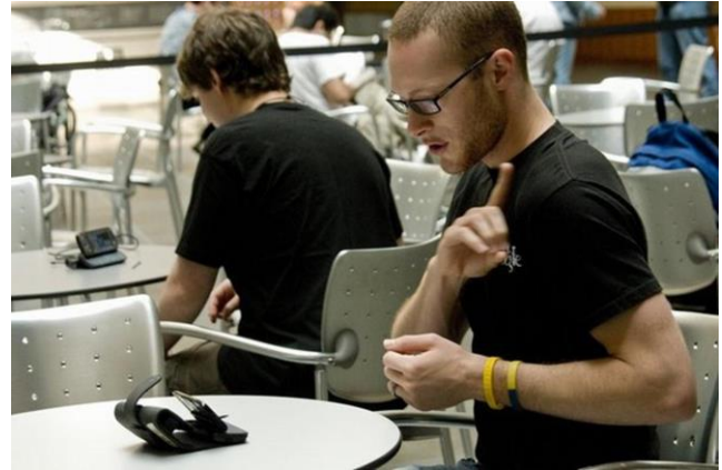
Figure 1: Two participants holding a real-time sign language conversation using the MobileASL software-providing real-time video at extremely low bandwidths (30 kilobits per second at 15 frames per second).
