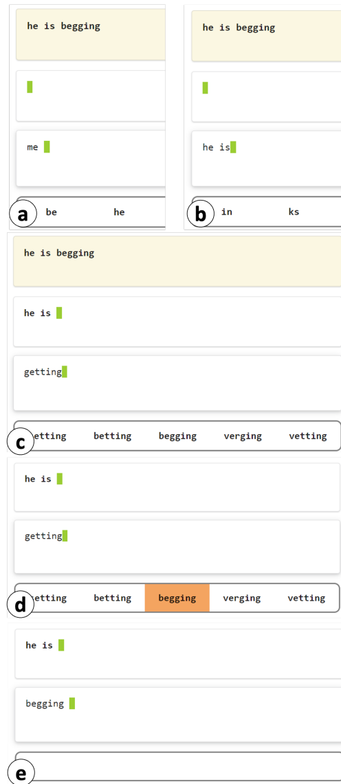
Figure 6: The typing flow of TypeAnywhere. The user is typing the sentence “he is begging” with the standard finger-to-key mapping. (a) After typing the first word, the decoder outputs “me” as the most probable text. (b) With more input context, the decoder is able to decode the tap sequence to “he is”. (c) The user first double-taps space to commit “he is” to the commit area , then types the last word decoded as “getting”. (d) The user then performs a selection gesture to trigger candidate selection and navigate to “begging”. (e) The word “begging” is now entered in the compose area after the user presses space.
