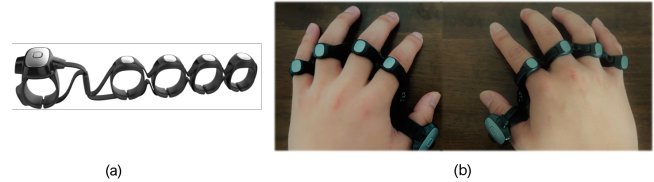
Figure 3: The hardware used in TypeAnywhere. (a) The Tap Strap device. (b) The user wearing two Tap Strap devices.
