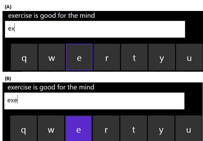
Figure 4. (A) When a user fixates on a key for at least 30% of its dwell time the border of the key changes color. (B) Once a key’s dwell timer is reached its background color is changed and the user hears an audible click.
