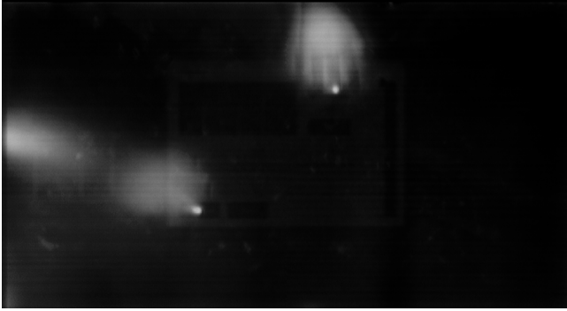
Figure 5. A raw image captured by Microsoft PixelSense on-board cameras showing two different people touching the screen.
