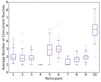
**Figure 4.** Distribution of the average number of concurrent touches per trial. Due to their touch behavior, participants impacted the screen with various parts of the hand, resulting in multiple registered touches.
