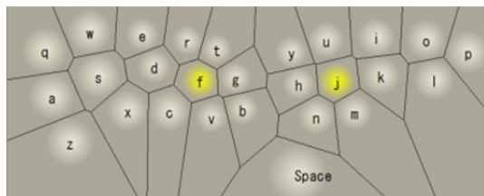
Figure 2. Visual adaptation of CATKey, showing Voronoi tessellation around adapted key centers (from [7]; copyright Springer).
