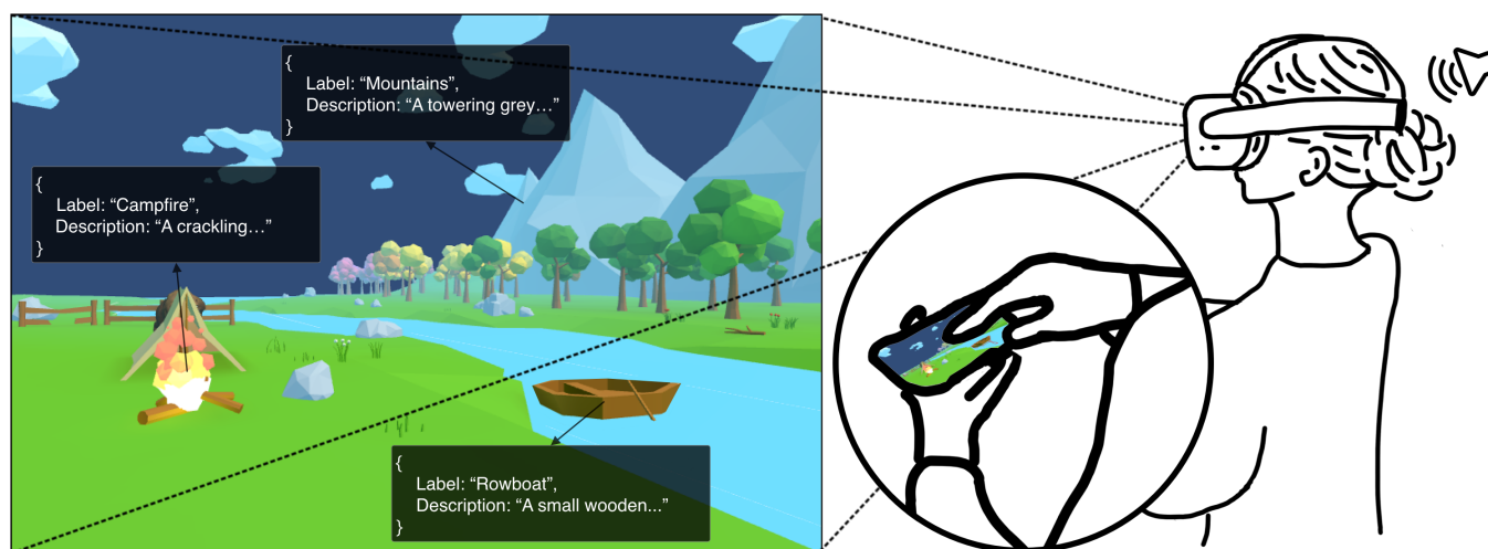
Figure 1: SceneVR is a touchscreen virtual reality (VR) controller that enables nonvisual access to virtual objects and avatars within a 3-D environment through a technique we introduce called “scene reading.” (Left) The virtual scene is a campground, where objects are annotated with labels and descriptions for a touch-based “scene reader.” (Right) The SceneVR touchscreen controller supports scene reading through touch gestures and spatial audio. SceneVR streams a real-time view from a VR headset to a user’s phone and lets them “read” the scene with their finger to identify virtual objects and avatars that they touch, similar to techniques used in Slide Rule [38], Apple VoiceOver, or Android TalkBack, but for 3-D scenes rather than 2-D interfaces.
