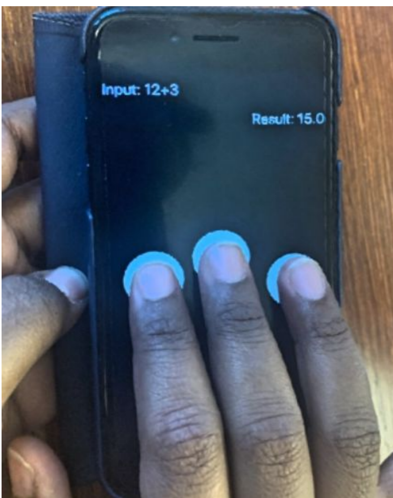
Typing "5" on GestureCalc. The gesture can be performed at any location on the screen.
