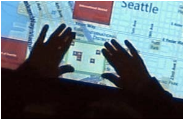
Figure 8. A participant uses both hands to hold a touchplate steady, causing some false touch events.
