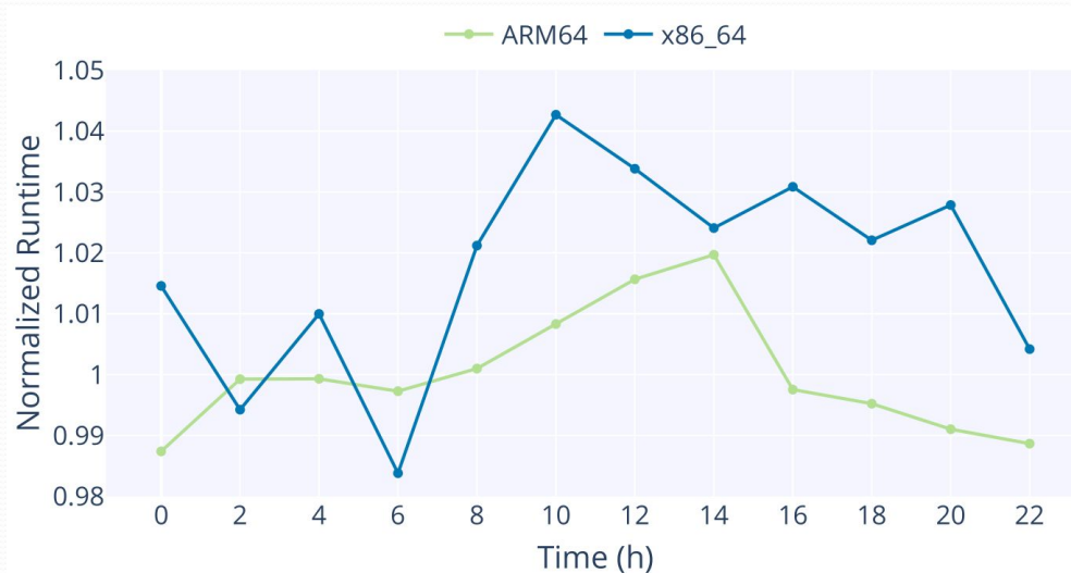
Global two-hour average NLP pipeline runtime normalized against global ARM64 average runtime
