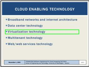
3. VIRTUALIZATION TECHNOLOGY Convert a physical IT resource into a virtual IT resource Servers, storage, network, power (virtual UPSs) Virtualization supports: Hardware independence Server consolidation Resource replication Resource pooling Elastic scalability Operating-system based virtualization Hardware-based virtualization TCSS462/562:(Software Engineering for) Cloud Computing [Fall 2022] School of Engineering and Technology, University of Washington - Taco November 1, 2022
