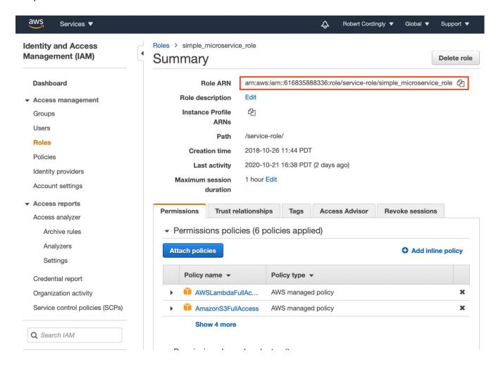
Copy your ARN shown at the top of the page. All functions can share the same ARN. Next open the **config.json** files located in each function's **deploy** folder and paste the ARN into the JSON attribute called **lambdaRoleARN**. **No other attributes in the config files need to be changed.**
