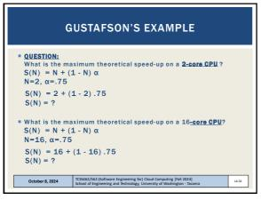
**GUSTAFSON'S EXAMPLE** • QUESTION: What is the maximum theoretical speed-up on a 2-core CPU?  $S(N) = N + (1 - N) \alpha$ N=2, α= For 2 CPUs, speed up is 1.25x S(N) =S(N) = ?For 16 CPUs, speed up is 4.75x What is the maximum theoretical speed-up on a 16-core CPU?  $S(N) = N + (1 - N) \alpha$  $N=16, \alpha=.75$ S(N) = 16 + (1 - 16).75S(N) = ?October 8, 2024 L4.32
