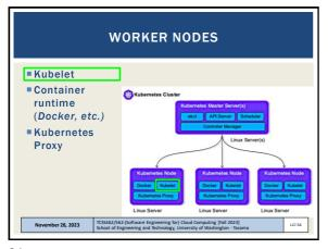
**KUBELET** ■ Main Kubernetes agent Runs on every node Adding a new node installs the kubelet onto the node Kubelet registers the node with the cluster ■ Monitors API server for new work assignments Maintains reporting back to control plane ■ When a node can't run a task, kubelet is NOT responsible for finding an alternate node ember 28, 2023
