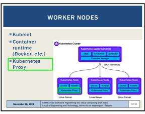
**KUBE-PROXY** Runs on every node in the cluster Responsible for managing the cluster's networking ■ Ensures each node obtains a unique IP address Implemented local IPTABLES and IPVS rules to route and load-■ IPTABLES (ipv4) - enables configuration of IP packet filtering rules of the Linux kernel firewall ■ IPVS - IP Virtual Server: provides transport-layer (layer 4) load balancing as part of the Linux kernel; Configured using ipvsadm tool in Linux November 28, 2023
