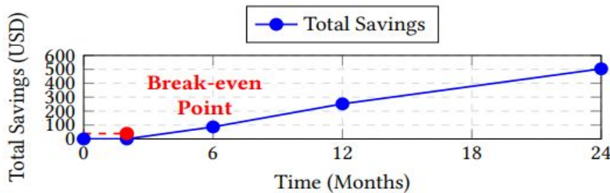
Figure 4: Projected cost savings over time, assuming 10 executions per day. The break-even point occurs at approximately 2 months.
