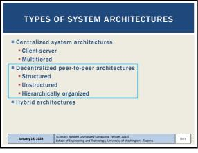
**DECENTRALIZED PEER-TO-PEER ARCHITECTURES** Client/server: Nodes have specific roles ■ Peer-to-peer: Nodes are seen as all equal... How should nodes be organized for communication? January 18, 2024 L5.72
