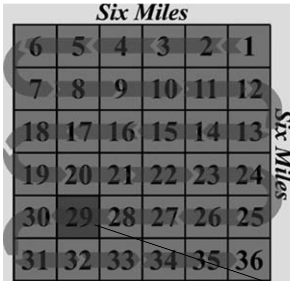
Figure 1-5A: The fundamental grid unit is a section , a 1 x 1 mile plot of land (640 acres), which are grouped into larger parcels of land termed townships . Each township is a 6 x 6 mile plot of land that contains 36 sections. Sections are numbered starting in the northeast corner of a given township as section 1 and then progressing sequentially in a zig-zag pattern ending in the southeast corner as section 36.
