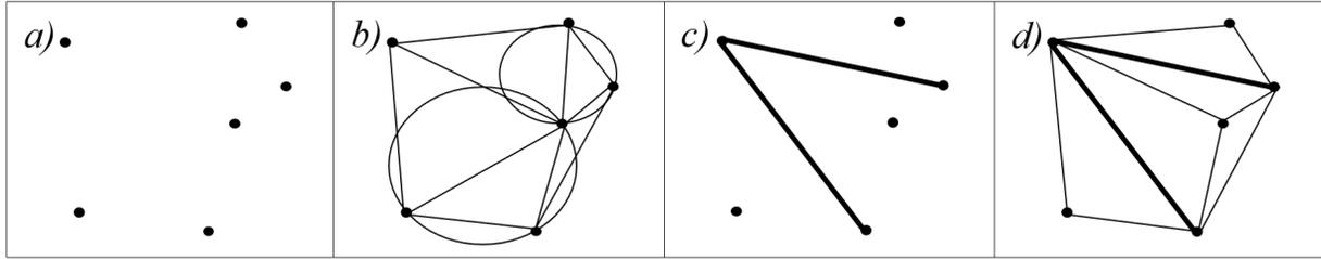
**Figure 6** (a) A set of vertices  $V$  and (b) its Delaunay Triangulation. (c) A set of vertices  $V$  and edges  $E$  and (d) its Constrained Delaunay Triangulation.
