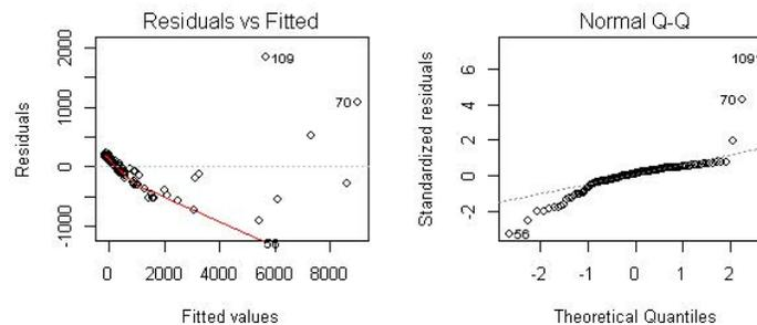
**Figure 13** Residuals and Q-Q plots for the linear fit of number of gate pairs versus total run time.
