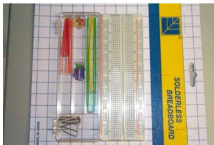
Figure 2 - Jumper Wire Kit with breadboard
