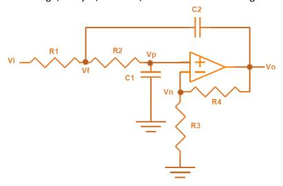
Figure 1. Basic Sallen-Key filter.
