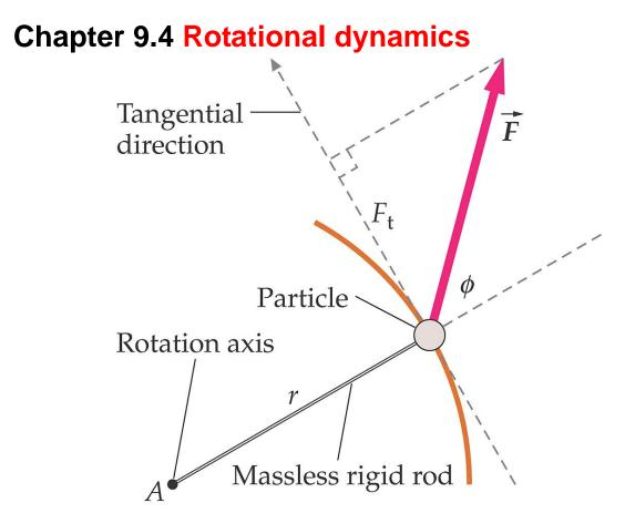
Particle of mass M pivots about axis thru A perp to the rod attaching it.
