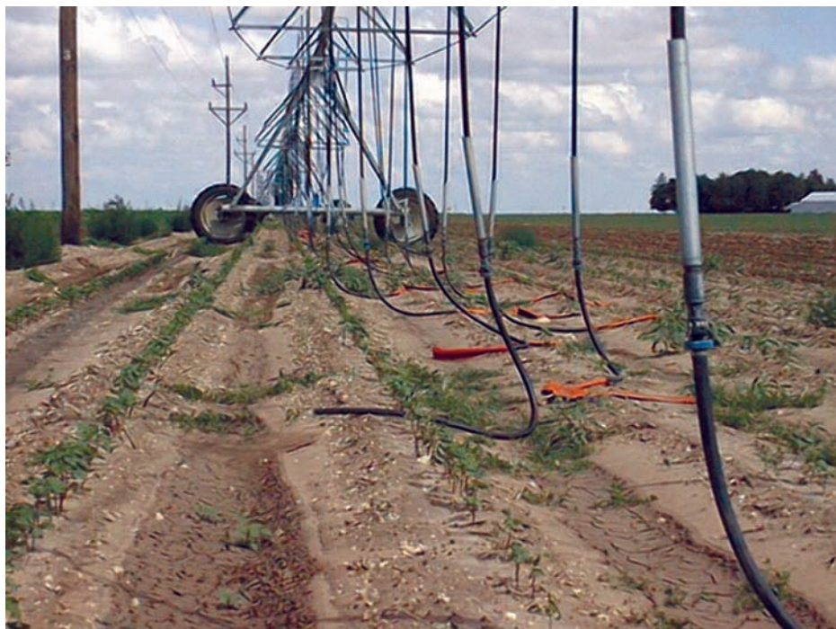
FIGURE 4-1 Low-Energy Precision-Application Irrigation System. SOURCE: USDA/ERS (2004).
