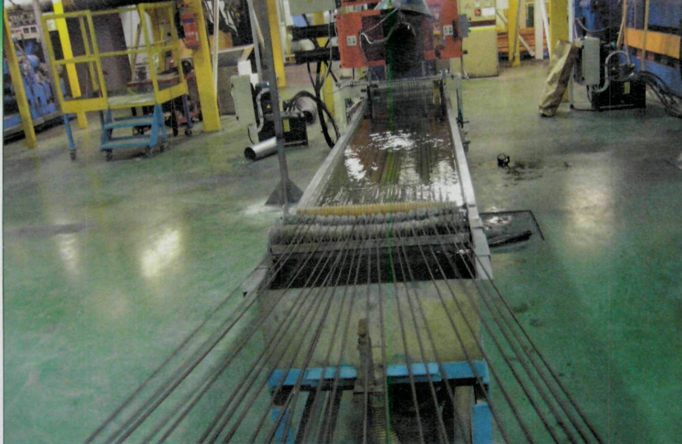
Axion's automated e-plastic recycling process separates polymers of low-FR materials like ABS from telephones.
