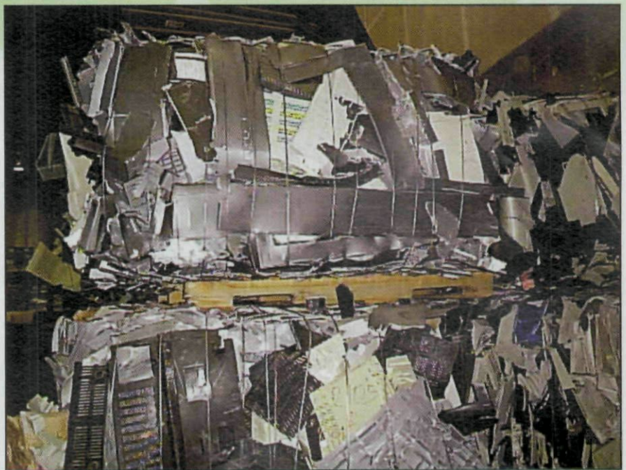
Plastics from old computers contain brominated FRs, making them unusable in Europe under new RoHS restrictions. (Photo: WM Recycle America)
