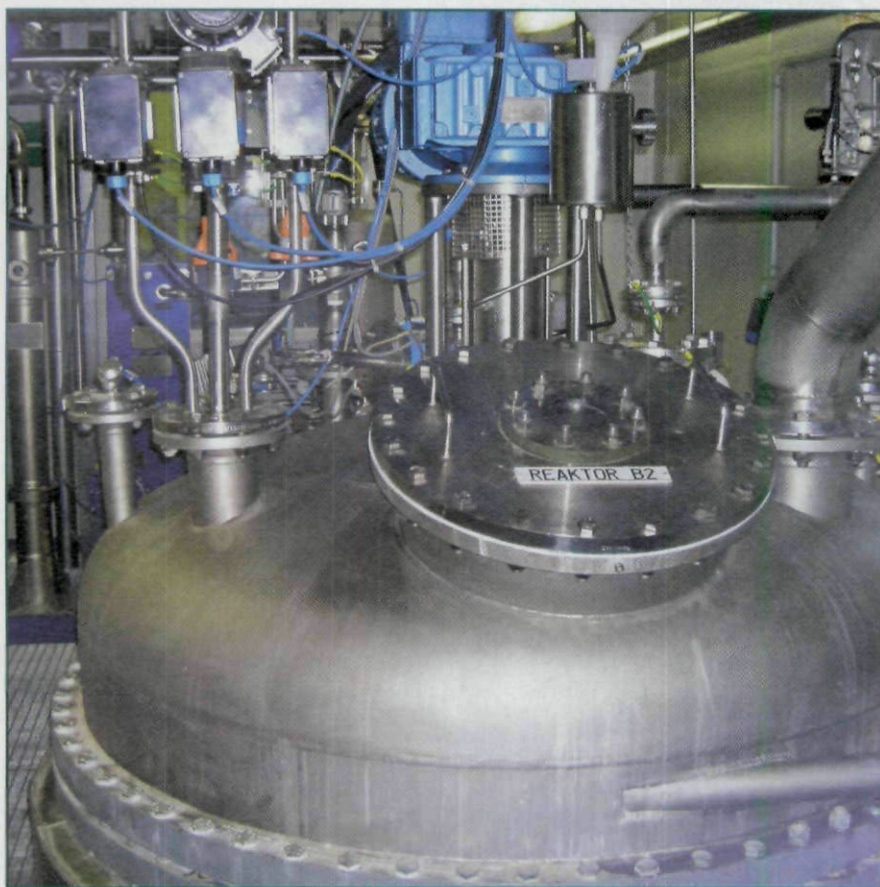
The Fraunhofer Institute's CreaSolv solution process produces clean e-plastics containing as little as 0.055% brominated FR. This tank is a pilot system.
