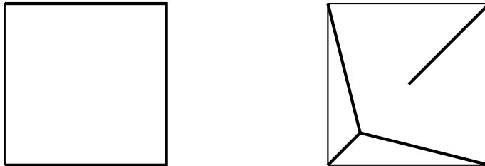
FIGURE 15. Left: three sides of the boundary give an opaque set with length 3. Right: the conjectured shortest opaque set for the unit square with length \sqrt{2} + \sqrt{3/2} \sim 2.63 .
