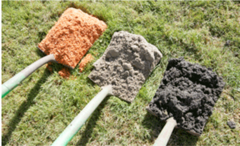
TAGRO Mix components: sawdust, screened sand and biosolids.
