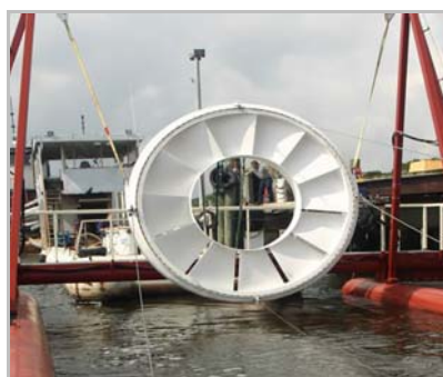
Figure 8. Open Hydro Rim Drive Turbine
