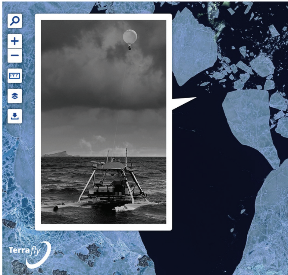
TerALTA balloon-mounted bathymetry sensor operated via a robotic vessel for NSF IUCRC Compendium CAKE-MSS Modeling Sea Surge and Flooding using ALTA and TerraFly
