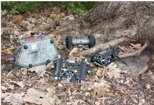
The Scout Robot Platform currently being used by the US Army and several police departments for search and rescue missions.
