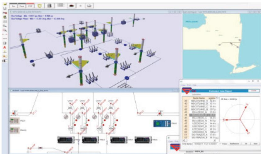
*The SuperCalibrator is a distributed state estimator that uses detailed models of substations and measurements from all substation devices to provide power operators with real-time information that can help them avoid blackouts and improve the efficiency of the grid.*
