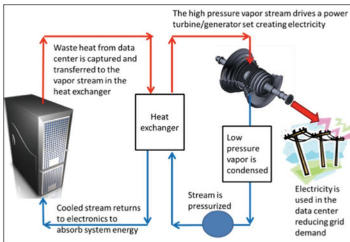
*An example of a waste heat power-producing cycle. The waste heat is captured from the data center and used as the heat source to boil an organic liquid. The high pressure vapor that forms when boiled spins a turbine, generating electricity. The low pressure vapor exiting the turbine is condensed, re-pressurized and the cycle begins again.*
