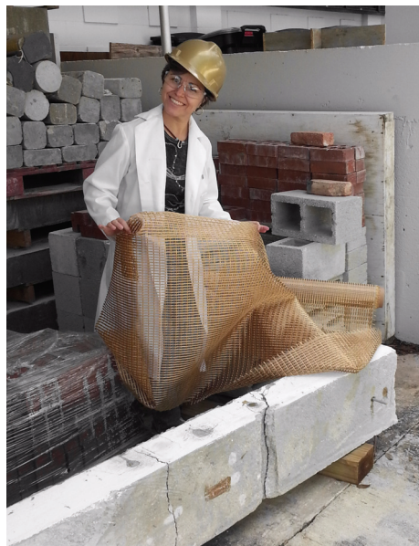
Fabric reinforcement for a concrete surface.
