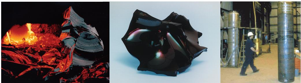
*Waste vitrification chemically processes heavy metals and radioactive elements into a durable, leach-resistant glass, which is then placed into a canister. Images courtesy of Pacific Northwest National Laboratory.*
