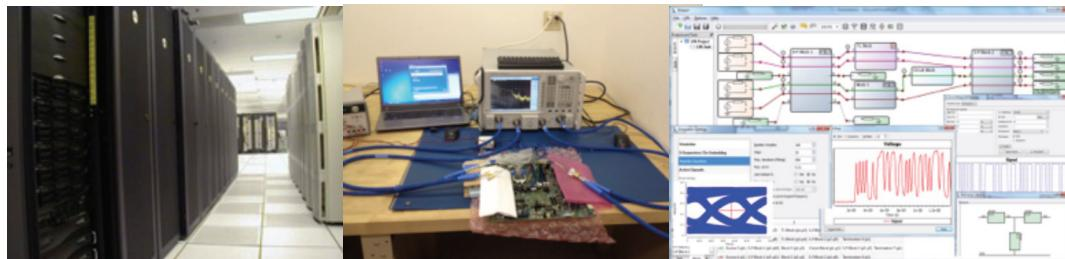
(Left) A massively parallel computing platform that uses high-speed links for data communication: an example end product that can benefit from the developed tool set; (Center) Laboratory measurement of a high-speed link: expensive instruments and expertise in high-frequency measurement are needed; (Right) A screenshot of the developed tool set for high-speed link-path analysis: cost-effective and no need for extensive training for the user.
