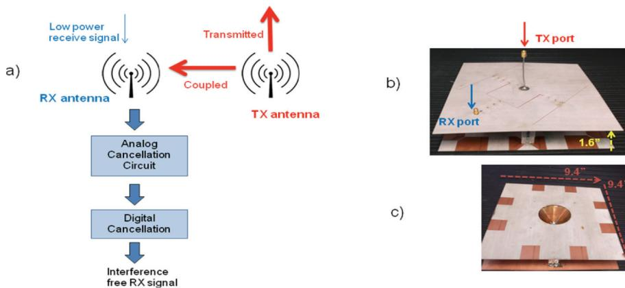
Above (a), a schematic view of the isolation problem between receive and transmit RF front ends; (b) Bottom view of the fabricated antenna and matching showing the RX and TX ports with integrated feed network; (c) Top view of the fabricated prototype.
