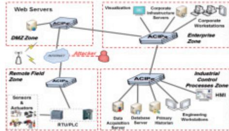
*Test bed based on Supervisory Control and Data Acquisition (SCADA) systems provides a platform for testing both hardware and software.*
