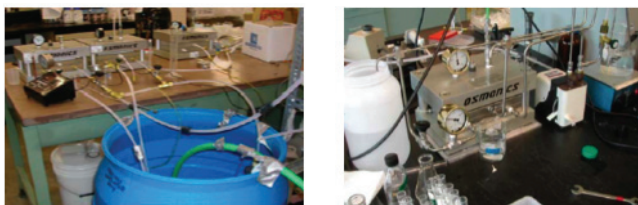
Above: Bench-scale experimental system for measuring membrane flux decline (left) and membrane rejection (right).
