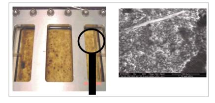
*Above*: Photograph showing the membrane surface after the onset of biofouling on the left; environmental electron scanning micrograph that shows the growth of the biofouling layer on the membrane surface on the right.
