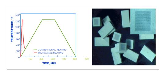
Left: Vastly improved production of base metal multilayer ceramic capacitors using microwave sintering techniques. Right: Examples of microwave sintered multilayer ceramic capacitors with nickel electrodes.
