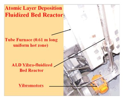
coatings of metal oxides and boron nitride particles. A patent has been filed, and a spin-off company, ALD Nanosolutions, has been formed to further develop the process and bring it to a commercially attractive level of performance. For more information, contact Professor William Koenke, 505-277-6824; e-mail: yonder@unm.edu.
