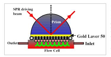
Understanding the short-term dynamics of interfacial processes is imperative in developing smart materials of the future. However none of the instruments allowed studying short term interactions in real time in situ. We developed a surface plasmon resonance spectroscope (adjacent figure) and applied it for the first time in studying the conformational dynamics of polymers and polymer surfactant interactions in millisecond time scales.
