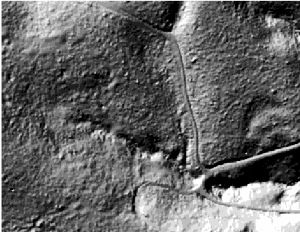
Figure 2: Lidar topography provides great detail, including streams, roads, ditches and slash piles. The upper right portion of the image has been harvested, while the rest is dense mature second growth.
