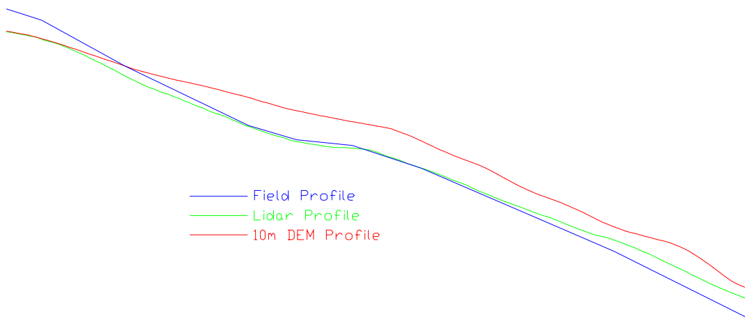
Figure 4: Skyline profiles from 1:4800 map (top), Lidar-generated profile and field data profile (both bottom). The Lidar profile
