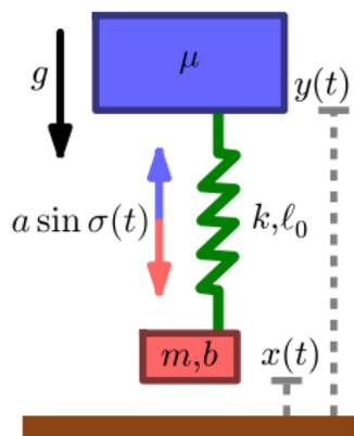
There exists a deadbeat control for vertical hopper, i.e. smooth actuator feedback law  $a(x, y, \dot{x}, \dot{y})$  such that hopper exactly tracks periodic orbit after one “hop”
