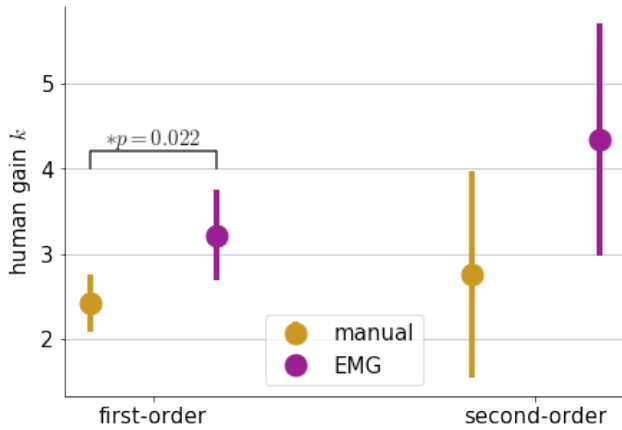
Fig. 5. The 95% confidence intervals for first- and second-order gain ( k ) estimates for manual (gold) and EMG (purple) interfaces. Lower values represent a smaller scaling factor. Statistically significant differences are marked with their respective p values.
