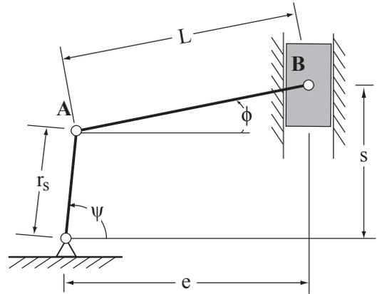
Fig. 4: Schematic of slider crank kinematics
