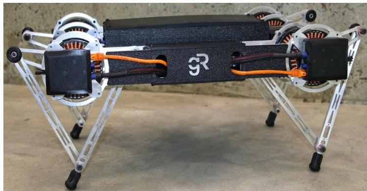
Figure 1.1. Four-legged Minitaur robot from Ghost Robotics
